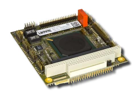
The Cool LiteRunner-LX800 is an affordable PC/104 single board computer, powered by an AMD Geode LX800 processor running at 500 MHz. It features 256 MB soldered DDR-RAM, AC97 sound and four USB 2.0 host ports. It is plug-in compatible to the familiar Cool LiteRunner 2, which has reached its end of life.
