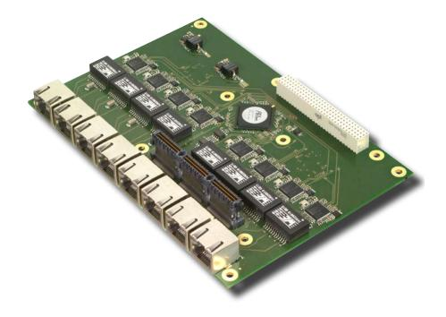
EXP-ETH9 is an eightfold Ethernet extension board for EPIC Express CPUs, which can also be used as a carrier board for PCI/104 Express processor boards.
