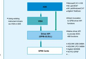
work with your applications in both ways. Its GPIB-32.DLL provides binary compatibility with the popular NI-488.2\* driver software. The USB-3488A and LPCI-3488A also provide VISA library support that can be used with most common instrument drivers written by instrument vendors. Regardless if you are using VC++, VB, Delphi, LabVIEW<sup>™</sup>\*, or any other T&M ADE, ADLINK GPIB interface cards are the most cost-effective GPIB solutions compatible with all your applications.
