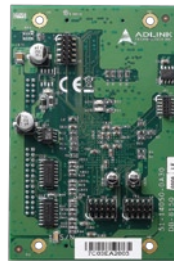
DB-8150 High-speed trigger
