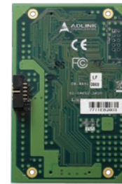
DB-8151 HSL bus distributed motion & I/O
