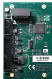
DB-8152 ECAM slave motion control
